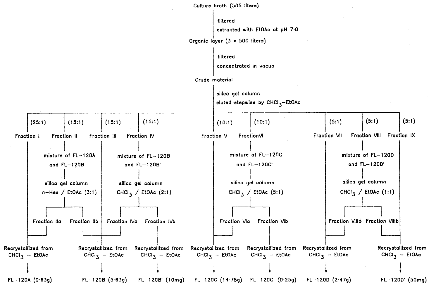
Fig. 2. Isolation procedure of FL-120A ~D' (1~6) and kinamycin D (7).
